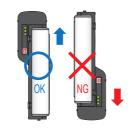
Examples illustrated as NG can lead to product failure by allowing oil to enter into the Winding Case in oily environments.
