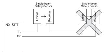
4. The total wiring length for the E3ZS Single-beam Safety Sensors is 30 m max.
