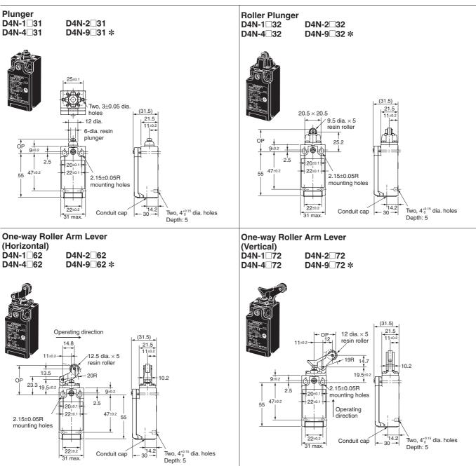
**Note:** Unless otherwise specified, a tolerance of  $\pm 0.4$  mm applies to all dimensions. \* Refer to page 12 for details on M12 connectors.
