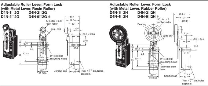
**Note:** Unless otherwise specified, a tolerance of  $\pm 0.4$  mm applies to all dimensions. \* Refer to following diagrams for details on M12 connectors.
