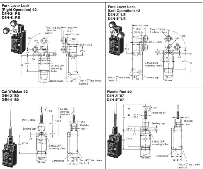
Note: Unless otherwise specified, a tolerance of ±0.4 mm applies to all dimensions.
