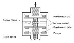
Conforms to EN60947-5-1 Direct Opening Operation  $\bigcirc$
