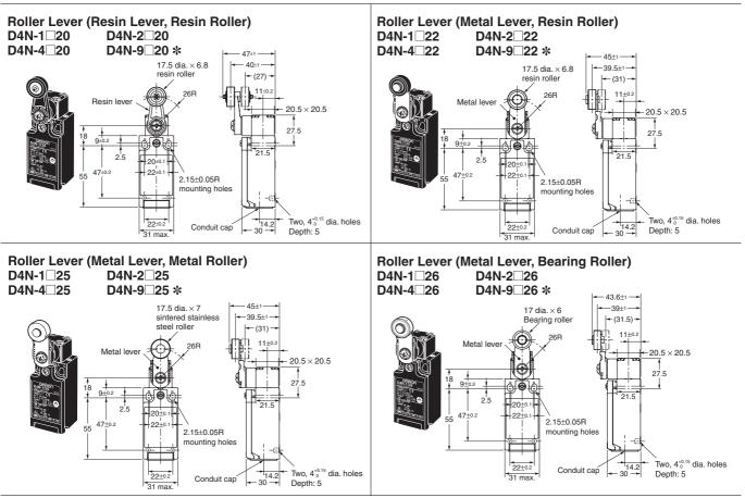
**Note:** Unless otherwise specified, a tolerance of  $\pm 0.4$  mm applies to all dimensions. \* Refer to page 12 for details on M12 connectors.
