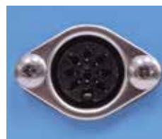
Remote cable entry on dust collector side
