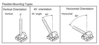
4. Using a shaft with an XY joint enables detection from above the production line.
